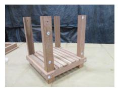
3. Flip the top upside down. With the legs assembled to the shelf, orient the legs so B1-B4 line up with the corresponding B1-B4 on the top. Once all the numbers line up, slide the legs into the frame on the top. You may have to flex the legs in slightly.
