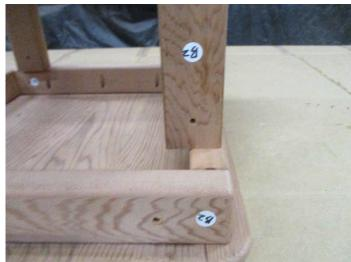
4. Once the legs are resting on the top, slide in the 4 carriage bolts into each hole on the top frame into the legs. The hole next to A1-A4 Put a nut and washer onto each bolt and tighten them down with a 7/16" wrench, 7/16" socket and rachet or an adjustable wrench. Once all the bolts are tight put a decorative bolt cap on the end of each carriage bolt.
